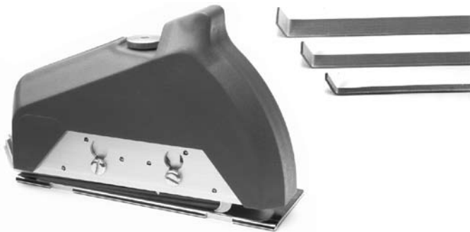
T103 Forbo Seam and Strip Cutter: Designed to score and trim the factory edges of linoleum products, leaving the appropriate bevel (undercut) easily and accurately in one step. It can be adjusted to any gauge of material from 2.0 mm up to 6.0 mm. It comes with three spacers to trim 10, 15, 20 or 30 mm strips. It uses Straight or Hooked Blades.
