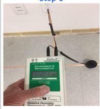
Test your grid as you go. The resistance to AC electrical should be less than one k ohm if using a megger. If using a standard volt ohm meter the readings are normally less than a few ohms.
