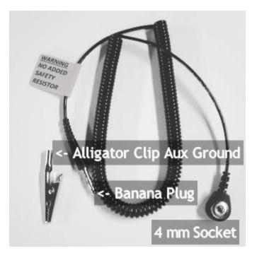
The GCNR-104MB consist of a 4 mm female socket securely attached to a 10' (fully extended) insulated curly cord that is terminated with a standard banana plug. This unit may be used with or without the alligator clip that is included with the assembly. The banana plug or the alligator clip (slipped over the banana plug) must be attached to a functional, reliable ground point as determined by the user.
