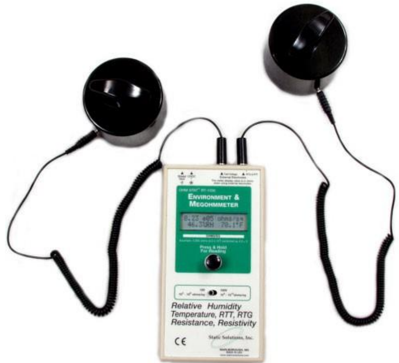
Figure 4 - Ohm - Stat RT-1000 Point to Point (RTT) test.
