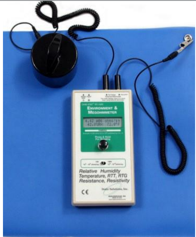
Figure 5 Ohm Stat - RT 1000 Point to ground (RTG) test
