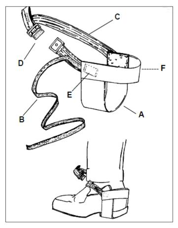
United SCP's High Visibility ESD Heel Straps feature colors that make it easy to see who is wearing their straps – and easy to see who is NOT! Adjust the tension one time and the quick release feature maintains the setting, making the straps easy to put on and easy to remove (no need to adjust the tension each time). They are non-marring, fit almost any style of shoe, and have a textured flooring contact surface for outstanding slip resistance.
